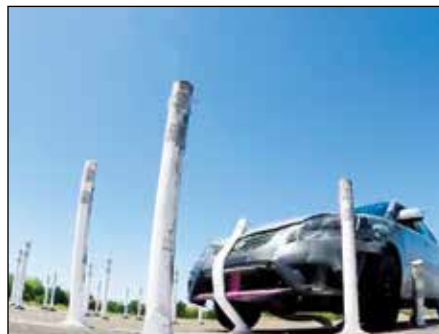
City Posts rebound to vertical, even after 100 hits at 70 mph
